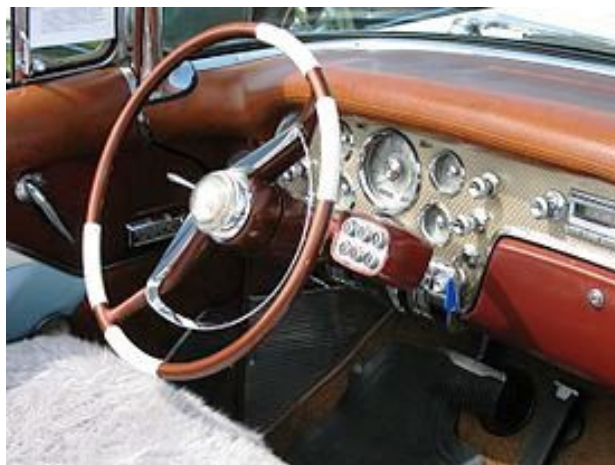
The column-mounted push button selector box for the Touchbutton Ultramatic in a 1956 Caribbean.
