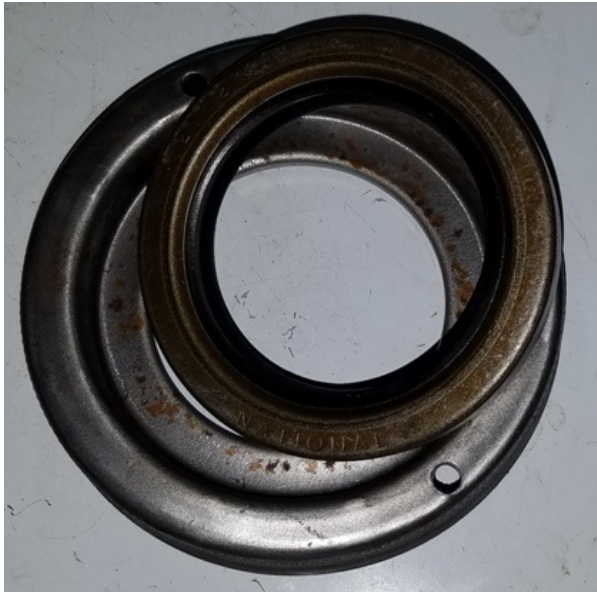
Front Crank Seal, in the timing cover. Note the two holes in the retainer, which align with two holes drilled through the timing cover, for installation of screws and nuts
