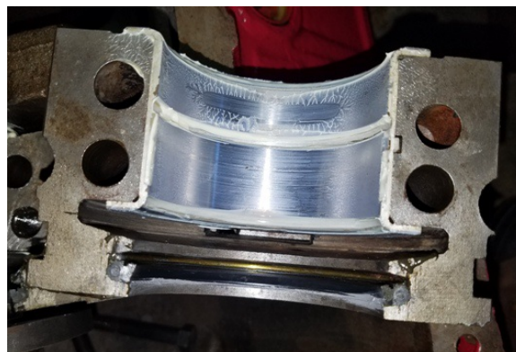
With the rear main seal, one pic shows it in place with the wire spacer installed alongside it.
