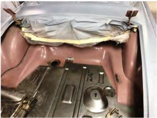
This is the trunk with the floor panel installed.
