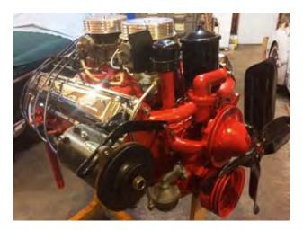
The engine is finished (a dual-quad 374 with all Jet-Streak components), Transmission is finished, Interior is finished but not installed, Twin-Traction 3.92 rear end is finished, fuel tank and radiator are done, new stainless exhaust is ready, but I haven't begun body and paint work at all, so none of those spiffy parts can yet be installed! Soon I hope.
