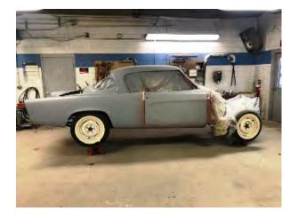
The new trunk floor is from Classic Enterprises. Next week, we should add final primer color to trunk. The final color should be on the car by Christmas. I also sand blasted and primed all Jack parts this week and the generator looks brand new. All gauges are being re-faced next week. Shouldn't be too much longer.
