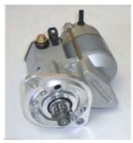
This starter has about 50% more torque and draws less amps during cranking. It weighs only 8 pounds, the original weighs about 17 pounds. This Starter has a built in Solenoid. It will hook up just like the original.
