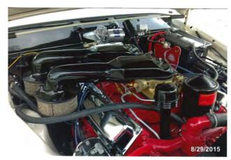
"The part that attaches to the carburetor appears to be the same as the standard oil bath, but once the narrow area is reached, the material is aluminum and is only about 3-4 inches in diameter."
