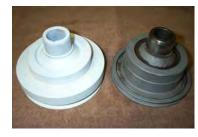
Note, the harmonic balancer in white primer is out of a 56J engine. The unpainted harmonic balance is the harmonic balance that just came out of my 56J with dual 4's, 3spd and overdrive car. The 56J red-orange paint has been stripped off.
