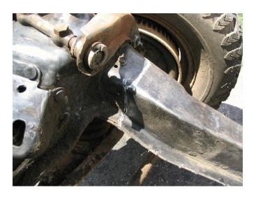
I thought I would mention to you, while cleaning the front frame, I noticed a substantial crack on the right member about 2-3" back from the front crossmember. It is not because of any rust as there isn't any, wondering if this is a common problem? It starts at the bottom of the right rail, goes up and across the top, where it stops. It is an easy welding repair, now the engine is out.
