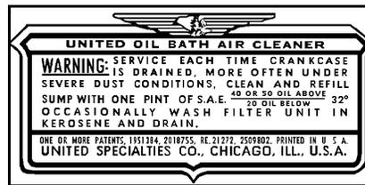
I was finally able to get the air cleaner (oil bath) decal reproduced. This is the decal with the special wording we have
